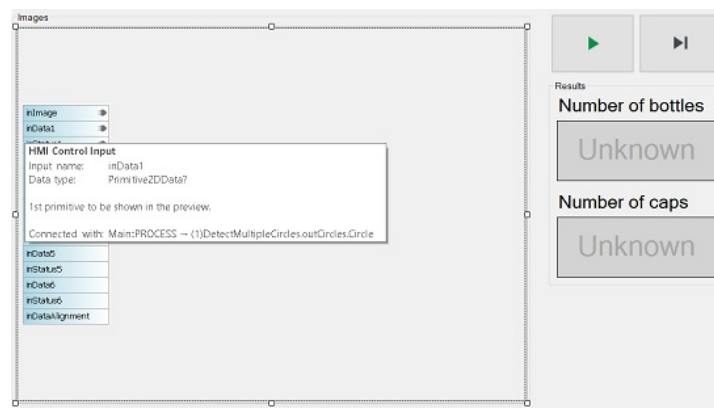
HmiView2DBox_PassFail used in the bottle crate example.
